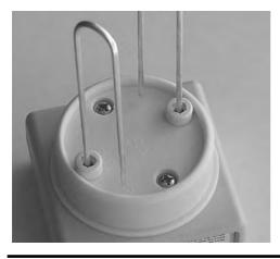
Insert the long end of silver electrodes into the sockets on the bottom of the generator. (You may need to push quite firmly). Rotate the electrodes so they are roughly parallel vertically and horizontally as pictured.
