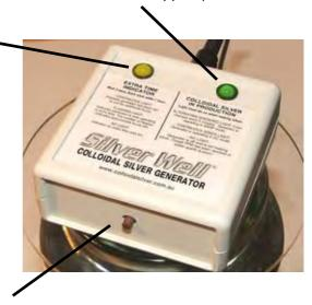
This switch adds EXTRA TIME that will commence once the Auto mode has completed its cycle. Each click adds 1 hour. You can add extra time any time the generator is operating with the right hand light illuminated. (To use the generator in IMPURE WATER you MUST add EXTRA TIME before the electrodes are lowered into the water. See page 9 for more in this).
